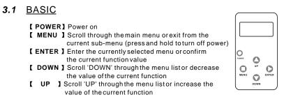
Note: The DMX Coder will automatically power off after extended periods of beingidle (1 minute)
