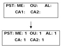
**Example:** Setting the unit to generate an Alert Message, call the administrators, generate a pulse (+V) and sound the audible alarm when PSTN failed.
