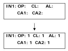
**Example:** Setting the input 1 to generate an SMS, call the administrators and sound the audible alarm when it triggered.
