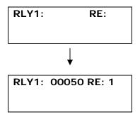
**Example:** To activate relay 1 to stay on for 50 seconds and with SMS reply from the unit after relay has turned off Simply input **000501**#
