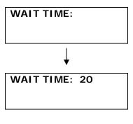
**Example:** To set the waiting time for 20 seconds Simply input 20 and ended with #
