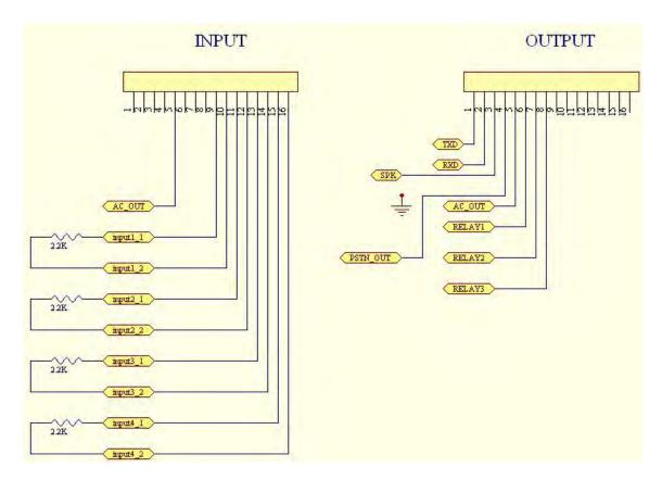
A 2.2K Resistor must be attached along with the sensors for all inputs
