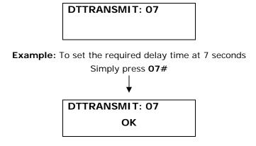
Note: The Delay Time is a 2 digits value range from 00 – 59 seconds (Default: 00 seconds)
