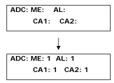
**Example:** Setting the unit to generate an Alert Message, call the administrators, generate a pulse (+5V) and sound the audible alarm when AC failed.
