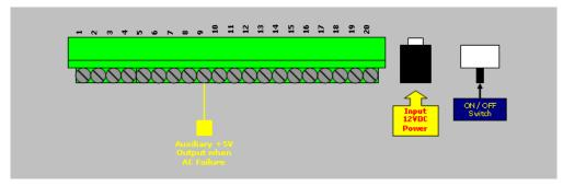
Note: Power Down Output facility can be used on alarm panel for alert notification
