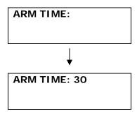
**Example:** To set the arm delay time for 30 seconds Simply input 30 and ended with #
