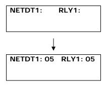
**Example:** To set the network failure time for 5 seconds and the turn on time of Relay 1 for 5 seconds
