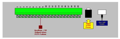
Note: PSTN Failure Output facility can be used on alarm panel for alert notification
