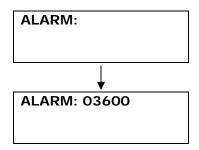
**Example:** To set the audible alarm to sound for 1 hour when triggered Simply press **03600**#
