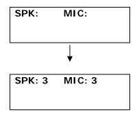
**Example:** To adjust the speaker volume to 3 and microphone volume to 3 Simply press **33**#
