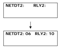
**Example:** To set the network failure time for 6 seconds and the turn on time of Relay 2 for 10 seconds Simply press **0610**#
