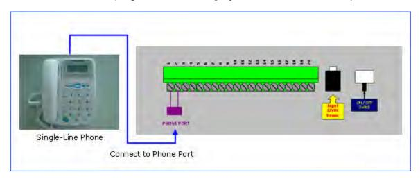
**Note:** Before commencing programming it is advisable to read the below programming setting instructions thoroughly. To start with programming, user must plug-in a normal single line phone to TEL1 (Port 1)
