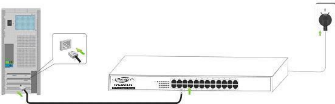
Figure 7. Connect a PC to the switch
