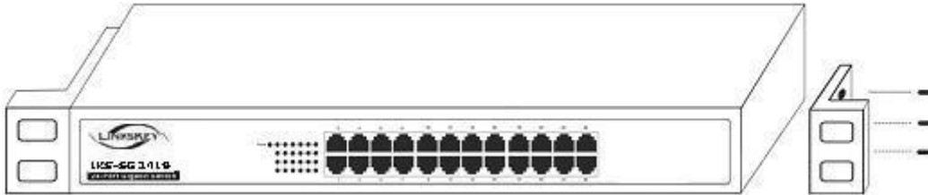
Figure 4. Attach L-shaped rack mount bracket to switch
