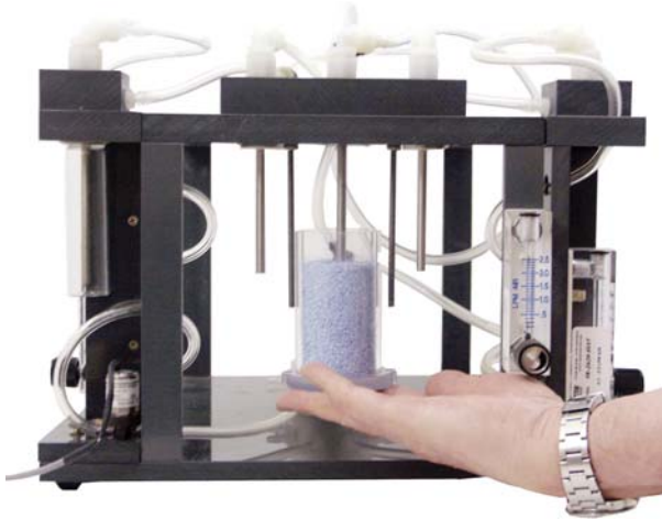
Figure 8 – Installing the Desiccant Container
