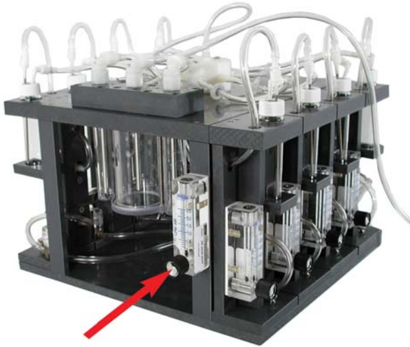
Figure 18 - Bypass Air Control
