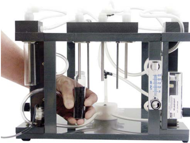
Figure 4 – Installing the Charcoal Filter Chamber
