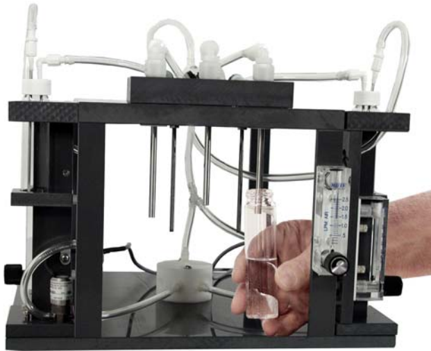
Figure 6 – Installing the Rehydration Chamber
