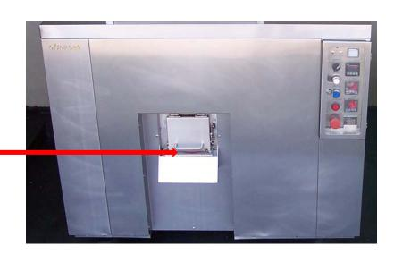
Then unlock the top input lid, fill the machine and start the cycle again
