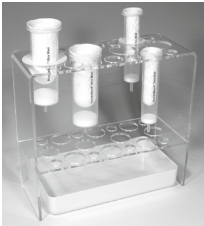
Figure 3: Setup of NucleoBond® Xtra Columns with the NucleoBond® Xtra Combi Rack A: Setup for clarification, loading, and first washing step; B: Setup for elution.
