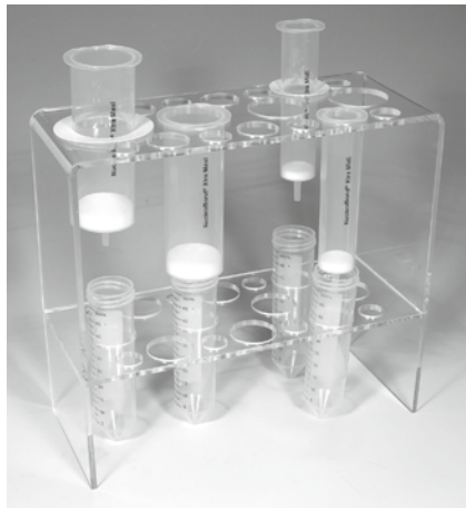
Figure 3: Setup of NucleoBond® Xtra Columns with the NucleoBond® Xtra Combi Rack A: Setup for clarification, loading, and first washing step; B: Setup for elution.
