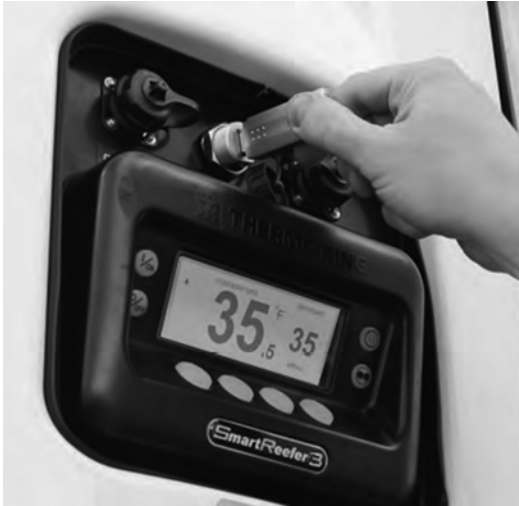
Figure 23: SR-3 HMI Control Panel
