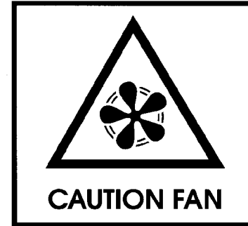
Figure 5: Fan Caution (Locations vary depending on model. Decals are located near areas that contain fans which can cause severe injuries when unit automatically starts.)
