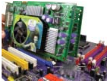
Installing two graphics cards
