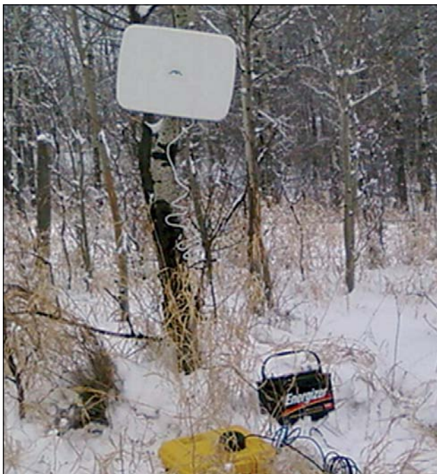
Use of Wifi for seismic system control and data retrieval, 2001 (SSC archive).
