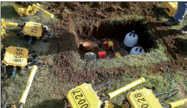
Sensor testing with Wifi pass-by download.
