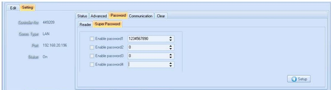
**Super Password:** Input super password from with Key pad Reader, the super password could access the DAC844 device directly without swipe any card. Each reader with only one super password and the maximum super password is 10 digit numbers.
