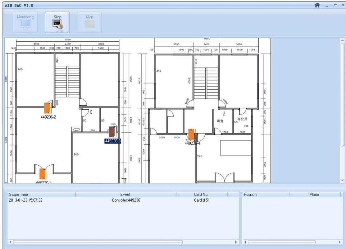
In the Real Time Monitoring windows, we can also support multiple records. Such as: Exit button open the door. Swipe the card to open the door. And the abnormality warning also display in the software. The abnormality warning will display in the right side of the Real Time Monitoring windows.
