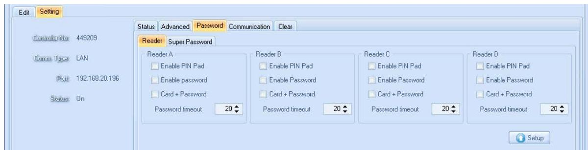
**Password:** Controls all of PIN Pad operation. Include enable PIN Pad, Super Password, Card+Password functions.
