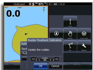
➔ **Note:** when centering the rudder during the calibration process, ensure the rudder is centered visually. The rudder feedback calibration dialog may show the rudder is centered (00 value) when the rudder is not centered. After centering the rudder visually, press **OK** and the rudder center calibration setting will be set to centered (00 value).
