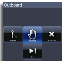
After the autopilot is engaged in NAV mode, the Autopilot controller will show NAV steering options.
