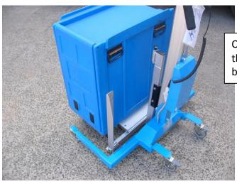
Once the trolley is correctly place underneath the road case, making sure that the case is stable before continuing. It is now ready to be lifted.
