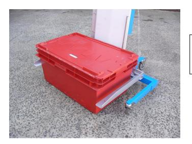
Once in this position the case is ready to be lifted, please ensure case is in proper position before continuing to the next step.
