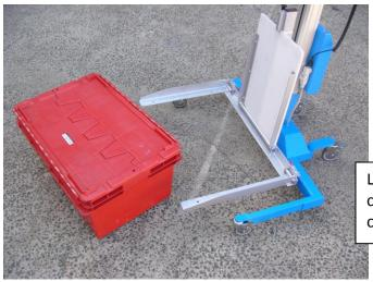
Lower forks below rim case, as the forks pick the case up from the rim; make sure the case is lined up correctly before proceeding with the next step.
