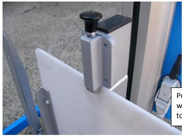
Pulling the tab located above the flat plate will allow the plate to be lowered in order to pick up the road case style loan sets.
