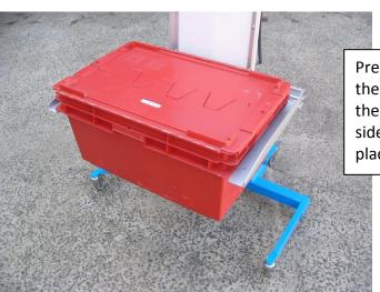
Press the button forwards to raise the case to the desired height, once at the correct height the Pronomic may be pushed forward, sideways or backwards to allow the case to be placed or unloaded in the appropriate area.
