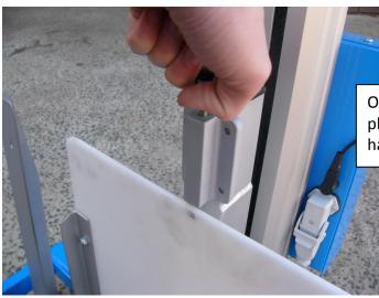
Once the tab has been pulled the flat plate will then have to be lowered by hand to its complete position.
