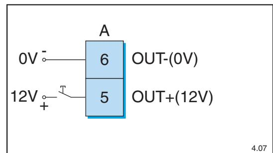
**i** The switching signal will be active for 30 to 35 ms, so that the drive can tighten the compression spring.
