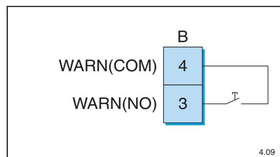
**i** The output contact (WARN) also closes when the RP600 is set to programming mode.
