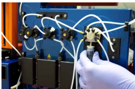
Figure 7.6: To remove the pump syringe the top screw must be turned counter-clockwise.
