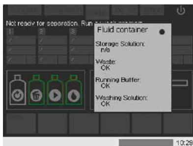
Figure 4.7: Fluid bottle status. By touching any fluid bottle symbol a pop-up box displays a text report of the fluid bottle status.
