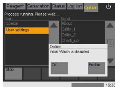
Figure 7.1: Initial wash program is used to activate or deactivate an automatic instrument prime on instrument startup.
