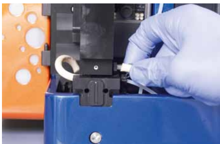
Figure 7.10: Remove the peristaltic pump tube from the washing station.
