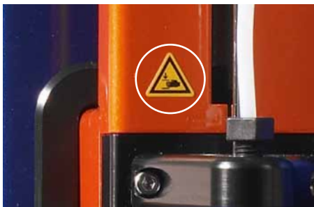
Figure 1.2: Open circle shows warning sign for hazard of crushing and shearing.
