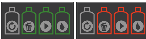
Figure 4.6: Fluid bottle status symbols. Left: Fluid bottles are ready. Right: Fluid bottles need to be replaced.
