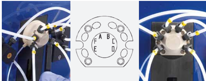
Figure 7.24: Connect tubing to the dilutor valve as shown above.
