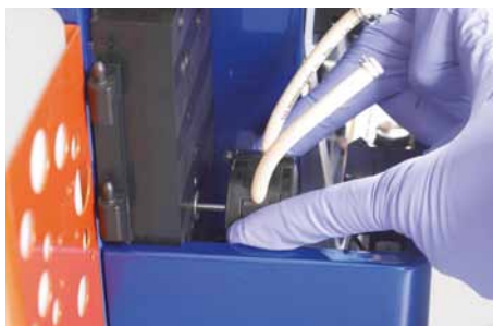
Figure 7.30: Detachment of the pump head.
