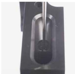
Figure 3.16: Test calibration of the needle arm position in the washing station.
