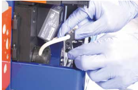
Figure 7.27: The waste distributor.
