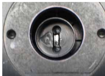
Figure 7.23: Inserting a new valve: take care to note the orientation of the valve.
