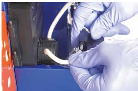
Figure 7.29: Disconnecting the tubing from the waste distributor.
