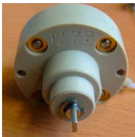
Figure 7.23: Inserting a new valve: take care to note the orientation of the valve.
