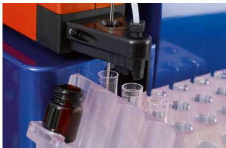
Figure 3.17: Test calibration of the needle arm position in the Chill Rack positions.
