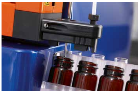
Figure 3.18: Test calibration of the needle arm position in the reagent vial.
