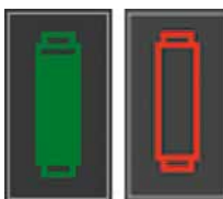
Figure 6.3: The column status graphic. Left: The columns are ready. Right: The columns must be changed.
