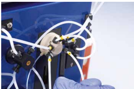
Figure 7.21: Unscrewing the tubing connected to the dilutor valve.
