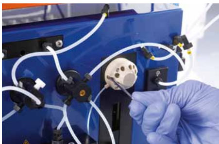
Figure 7.22: Unscrewing the dilutor valve's socket screws.
