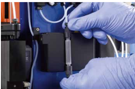
Figure 3.25: Removal of the column substitutes from the column slots.
