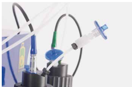
Figure 3.13: Positioning of the hydrophobic air filters on the bottle closures.
