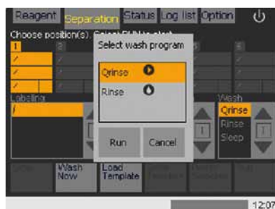
Figure 6.5: The "Wash Now" command displays two options: "Qrinse", for a quick rinse, and "Rinse". A full rinse is required for instrument priming.
