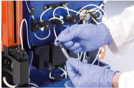
Figure 3.26: Unscrewing the top column connector for column removal.
