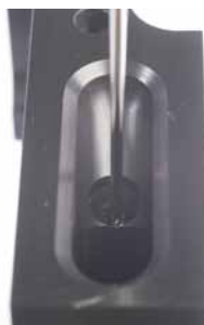
Figure 11.5: Test calibration of the needle arm position in the washing station. The position of the uptake needle should appear as shown above.
