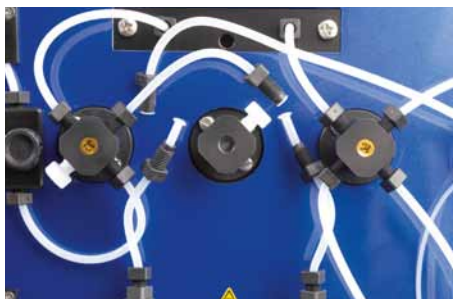
Figure 7.16: The valve cover-screw is unscrewed. Tubing and valve port locks or blind screws are detached.
