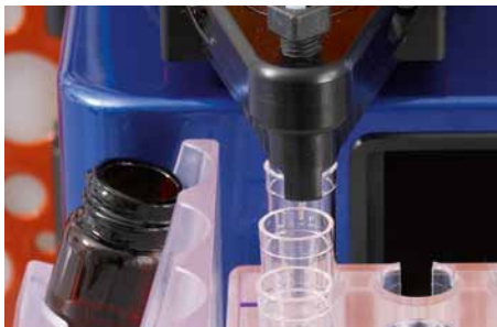
Figure 11.8: The uptake needle should be positioned as shown above.
