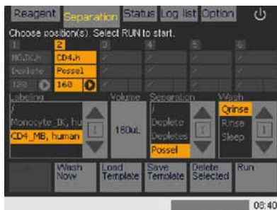
Figure 4.20: A sample template was setup to process two samples. Sample 1: Isolation of untouched human monocytes using the Monocyte Isolation Kit II, human (# 130-091-153); autolabeling program "MO.IK.h"; separation program "Deplete". Sample 2: Direct labeling and positive selection of CD4 + cells using CD4 MicroBeads, human (# 130-045-101); autolabeling program "CD4.h"; separation program "Possel".
