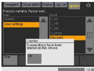
Figure 4.31: "Sepcount": viewing the number of performed separations. In this example, no separations have been performed using this instrument.
