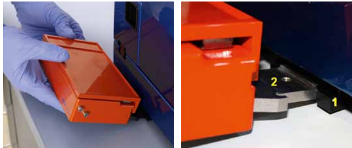
Figure 3.4: The receiving slot (1) and guide (2) of the MACS MiniSampler.
