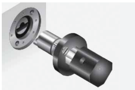
Figure 7.20: Inserting the new valve.
