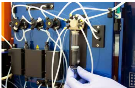
Figure 7.9: The plunger is placed in its fitting in the plunger holder. The plunger screw is fastened.
