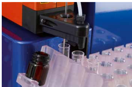
Figure 11.7: Calibrating the position of the needle arm in the sample tube.
