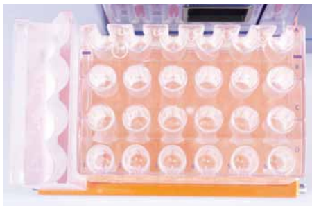
Figure 3.12: Positioning the Chill 5 Rack adjacent to a MACS Reagent Rack 4 on the MACS MiniSampler.
