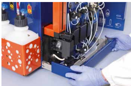
Figure 7.14: The bottom cover must be removed for access to the lower valve.
