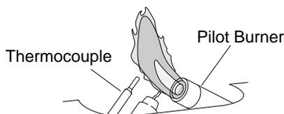
Figure 20 - Incorrect Pilot Flame Pattern
