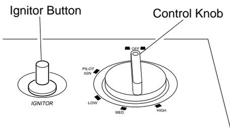
Figure 16 - Control Knob In The OFF Position
