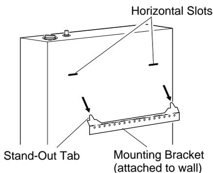
Figure 10 - Mounting Heater Onto Mounting Bracket
