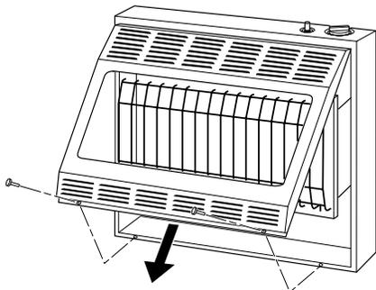
Figure 6 - Removing Front Panel Of Heater
