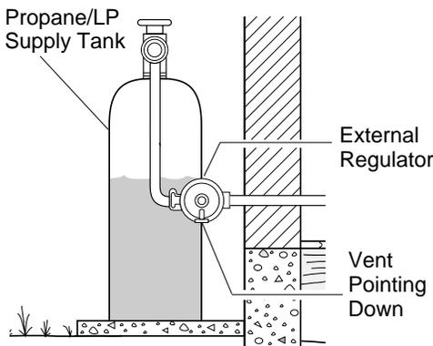
**Figure 12 - External Regulator With Vent Pointing Down**
