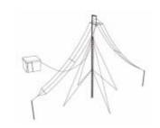
The Multi-wire Broadband Dipole Antenna is a 3-wire terminated folded dipole antenna designed for broadband operation. It is available in multiple power levels up to 1 kW.
