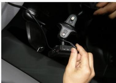
Connect external camera, GPS module, VIDEO OUT cable.
