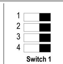
*The configuration of the parameters can be done either with the DIP switch or via software (you can not combine both solutions).*
