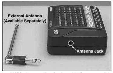
The 72MHz Frequency Checker has a built-in antenna which is designed to receive transmitter signals from within a 300 foot radius. If a greater range is desired, an external antenna is available separately (HCAP0341). Contact your local hobby shop for details. Using the external antenna can extend the Frequency Checker's range to a radius of 1000 feet. It's best to point the antenna skyward for best reception.
