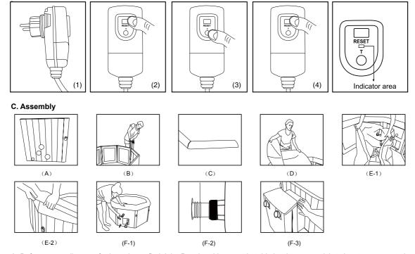
A. Before proceeding any further, please find Joint Panel and be sure that this is where you wish to locate your control box. The first side of the spa is where the control box will be connected and located. Also note, the Corner Beams shall face outward with the side including bluckle plate, and snap end is up, otherwise the assembly will be failed finally.
