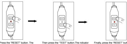
Press the "RESET" button. The indicator area should turn red.
