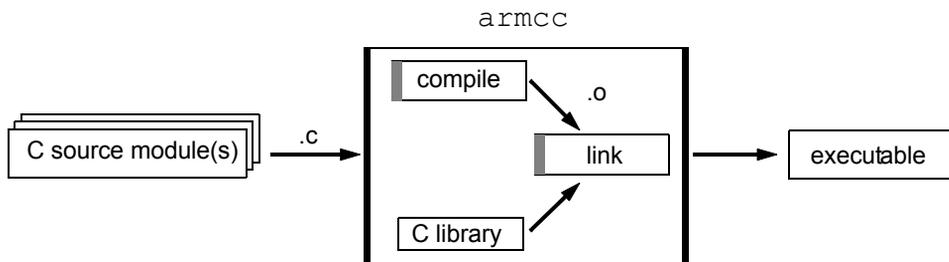
Figure 4-1 Compiling and linking C
