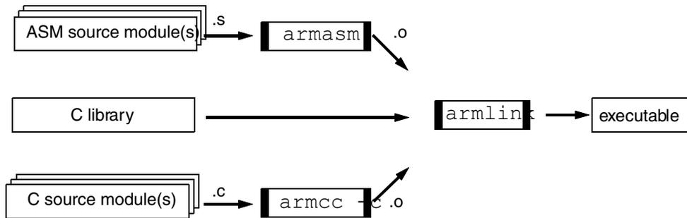
**Figure 6-1 Mixing C or C++ and assembly language**
