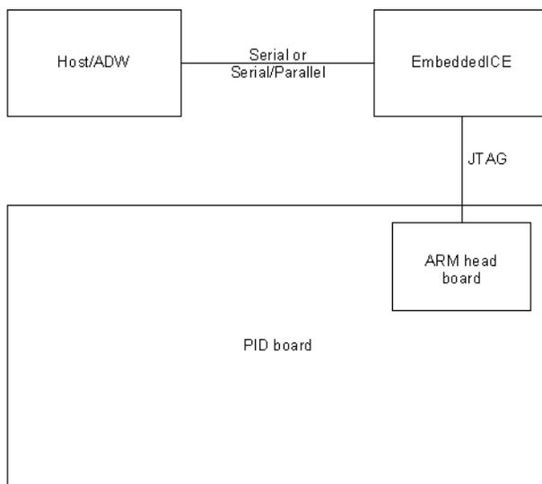
**Figure 3-1 A typical debugging set-up**
