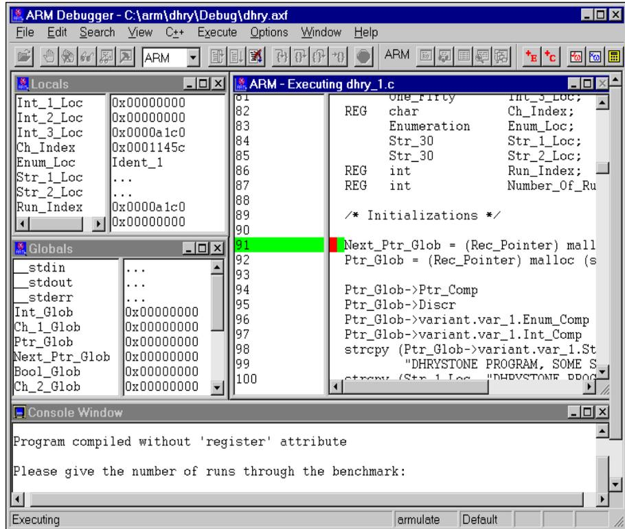
Figure 3-2 A typical ARM Debugger desktop display
