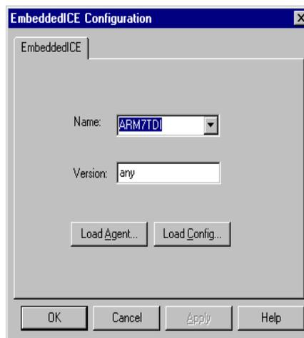
Figure 3-20 Configuration of EmbeddedICE target
