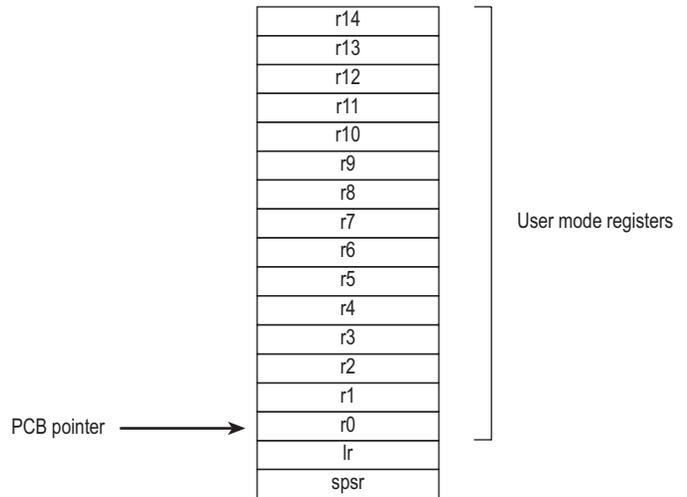
**Figure 9-3 PCB layout**
