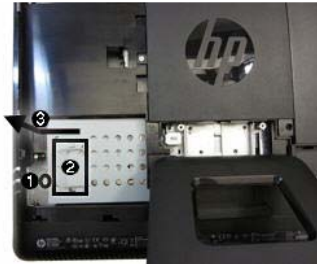
Figure 7-9 Removing the hard drive
