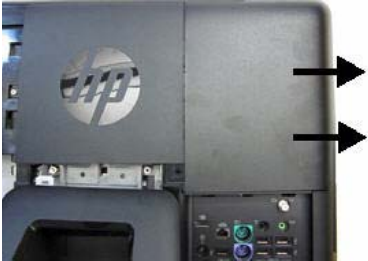
Figure 7-12 Removing the memory cover
