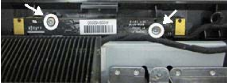
Figure 7-17 Removing the webcam module
