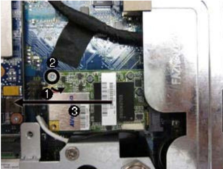
Figure 7-27 Removing the TV tuner module
