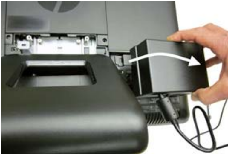
Figure 7-2 Removing the port cover
