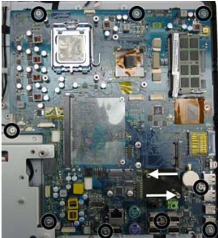
Figure 7-52 Removing the system board
