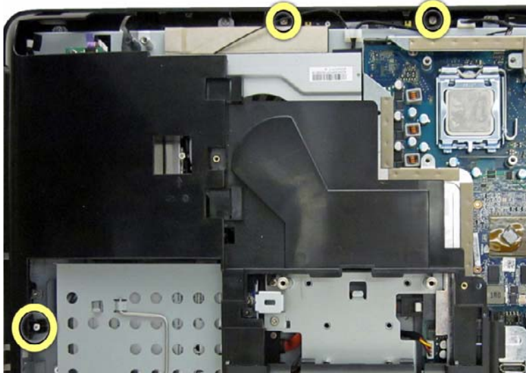
Figure 7-32 Removing the outer/left rear panel screws
