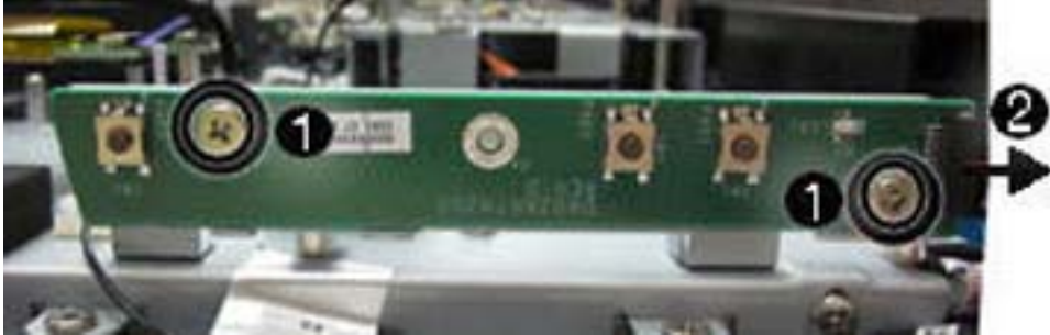
Figure 7-35 Removing the display control board
