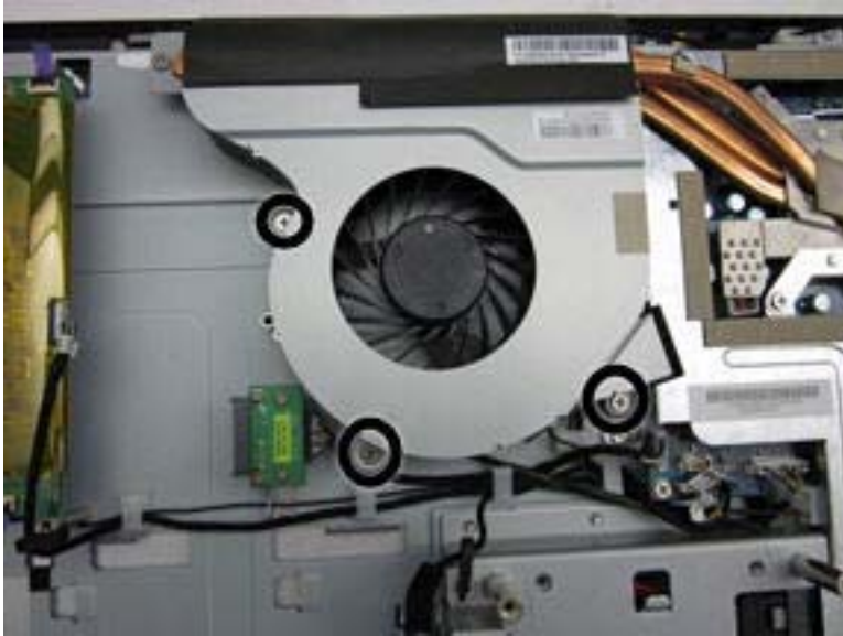
Figure 7-47 Removing the fan
