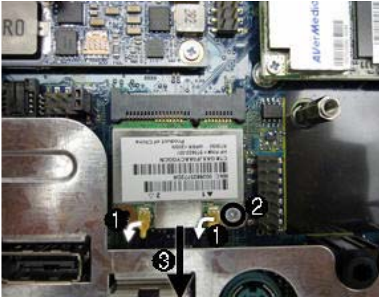
Figure 7-31 Removing the WLAN module
