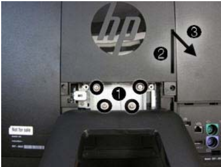
Figure 7-3 Removing the stand
