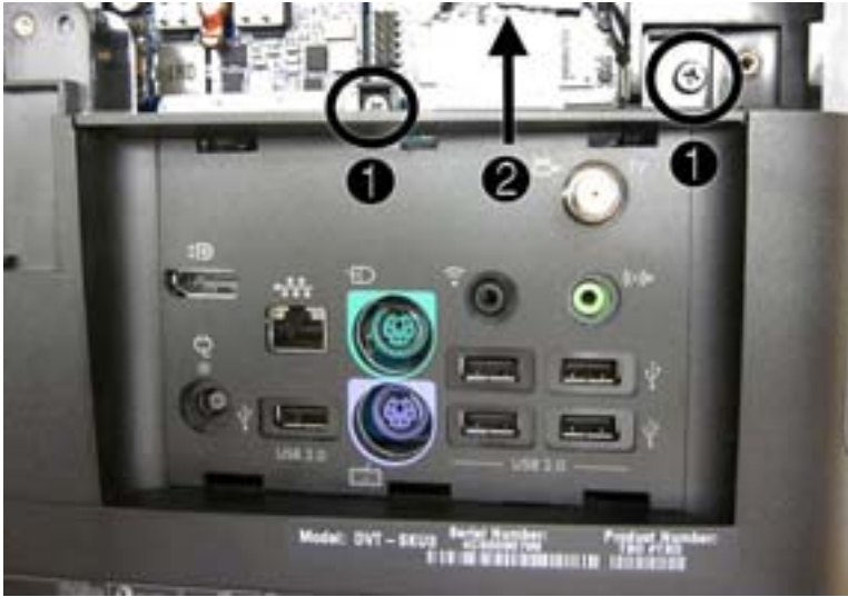
Figure 7-25 Removing the I/O panel
