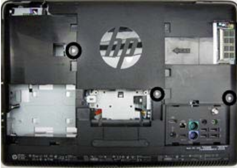
Figure 7-15 Removing the upper rear panel
