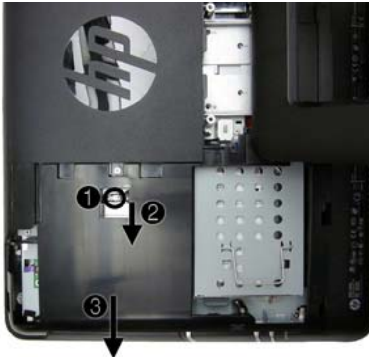
Figure 7-6 Removing the optical drive
