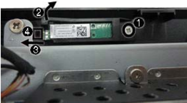
Figure 7-19 Removing the Bluetooth module
