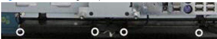
Figure 7-49 Removing the speakers
