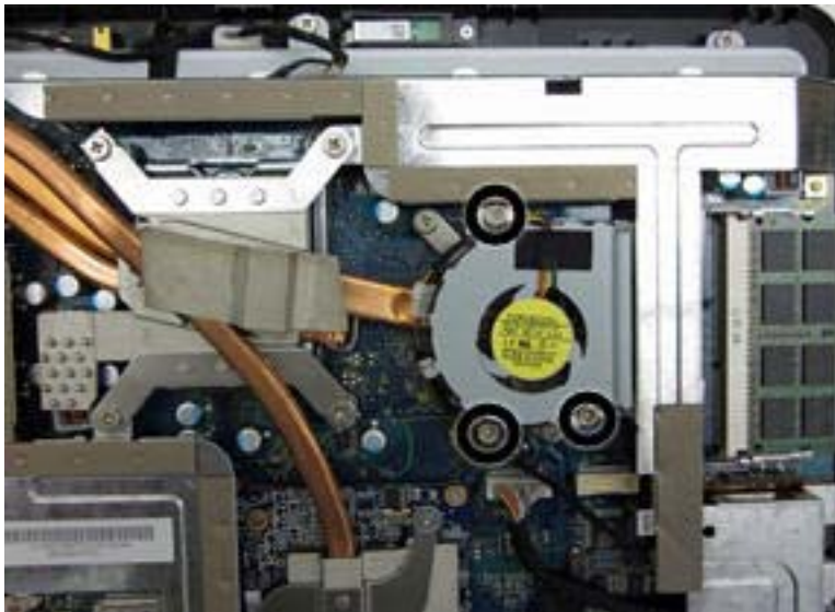
Figure 7-20 Removing the small fan
