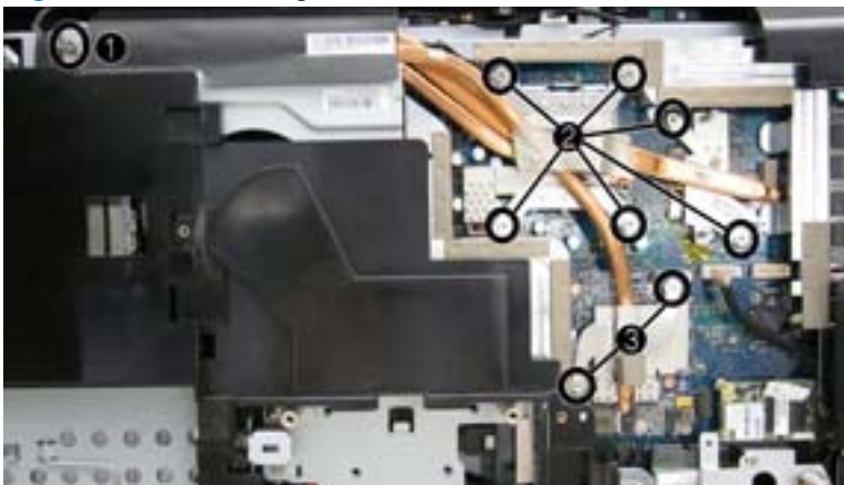
Figure 7-21 Removing the heat sink
