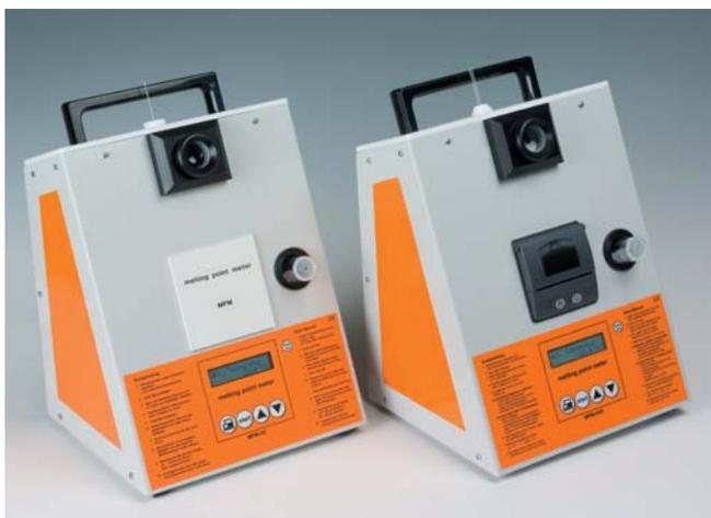
Ideal for determination of the melting point of powders and substances that do not have a clear transparent melting point.
