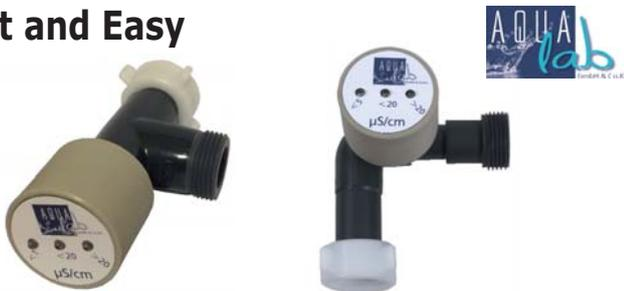
The 3D conductivity meter is battery driven to control the conductivity of pure and demineralized water. The scaled value can be controlled with three light-emitting diodes (LED) green, yellow and red. The limited values are available in two performances: <1, <20, >20µS/cm and <5, <20, >20µS/cm, and two applications: straight (illustration 1) and angular (illustration 2) The unit consists of a plastic housing with a R 3/4" connection.
