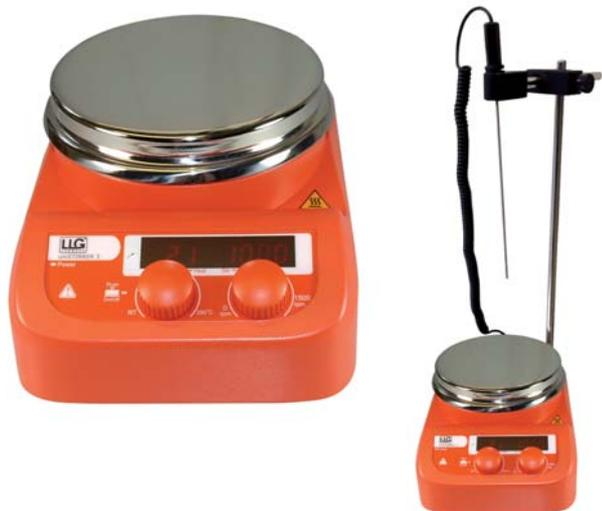
Cost effective magnetic stirrer with all essential functions and equipment features. A LED display to control all parameters, an integrated temperature control as well as an enclosed design (IP42) are integrated features. The included PT-1000 sensor ensures an exact temperature control. A stand rod with a sensor holder is supplied with this instrument. The integrated HOT-sign warns the user of a hot plate even if the device is switched off. 3 years warranty.
