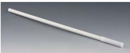
PTFE-encapsulated stirring bar retriever with strong permanent magnet (Alnico 5), universal chemical resistance. For the removal of stirring bars from aggressive liquids, prevents loss of stirring bars. Lower end diameter 10mm.
