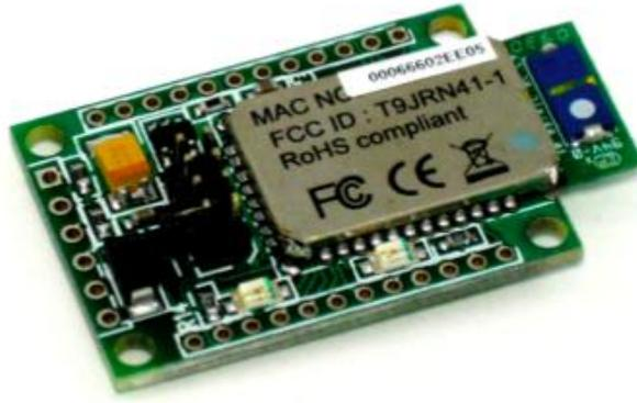
Figure 4.4 Roving Networks RN-41-SM
