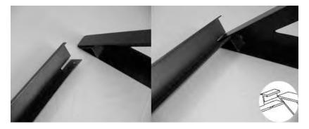
3. Slide remaining top support bar onto side triangle supports utilizing the stud/slot join.
