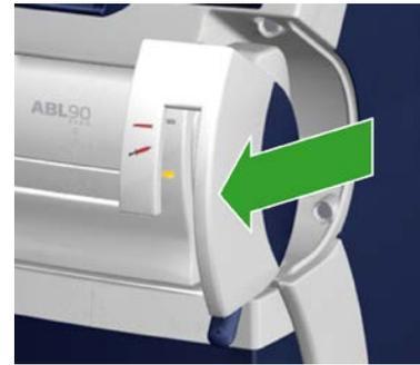
2. Lift the inlet handle to syringe position (the middle LED lights up).
