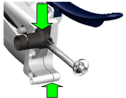
7. While pressing the two parts together, put the black inlet connector over the pin in the recess until a click is heard.
