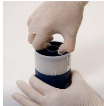
6. Remove the new sensor cassette by pulling it out of the sensor cassette pack with thumb and index finger.
