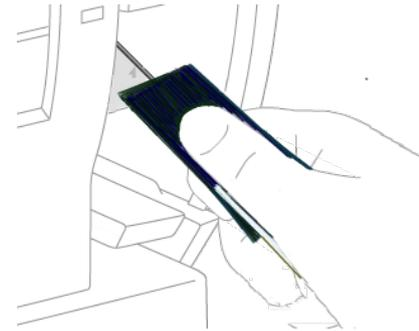
10. Push the adapter into the analyzer as far as you can and hold it there.
