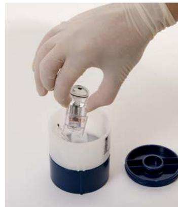
7. Holding the new sensor cassette with the thumb and index finger, press the new sensor cassette firmly into the sensor cassette seat in the sensor compartment until resistance is met.
