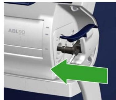
6. Put the inlet handle in the closed position and remount the cover.
