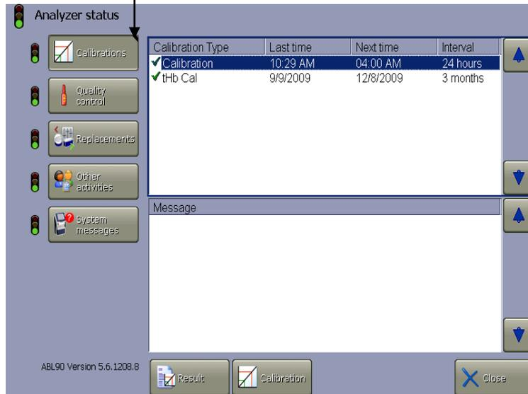
The traffic light color of the **Analyzer status** button is determined by the traffic light colors of the following status elements:
