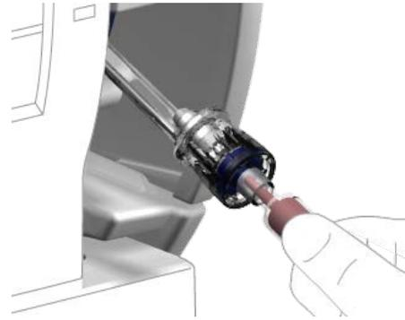
**NOTICE:** Be careful not to bend the probe. Hold on to the syringe barrel and do not press the plunger.
