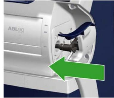
8. Put the inlet handle in the closed position and remount the cover.
