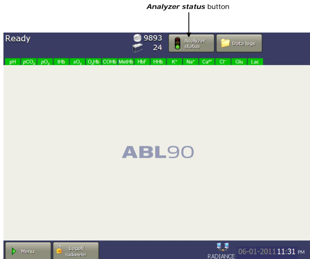
To enter the **Analyzer status** screen, press **Menu > Analyzer status** or press the **Analyzer status** button to access the analyzer status directly.
