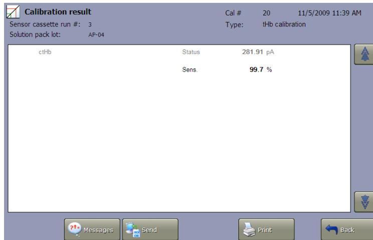
**Sens.** (cuvette factor) is a factor that expresses the ratio of the effective light path of the analyzer cuvette to that of a reference cuvette determined by Radiometer.
