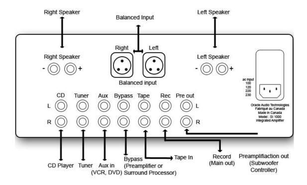
The Oracle SI 1000 is equipped with four (4) Unbalanced inputs (RCA) and one Balanced input (XLR). For optimal results we recommend the use of Balanced connections whenever the source component is equipped with a Balanced output.
