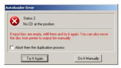
There are no discs in input bin, so autoloader reports it can't find CD at this position. You have now 2 possibilities. Refill input bin with empty discs and try it again or you can also put disc in appropriate recorder manually. If you check "Abort the duplication process", it will work like if you click Stop button from toolbar after solving this error.
