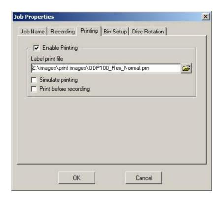
The following option *Bin Setup* will be enabled only if you have your autoloader configured with individual control of its bin. Then you can set which hopper is for your job input and which is output.
