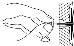
Figure 13 - Popping Open Anchor Wings For Thin Walls
