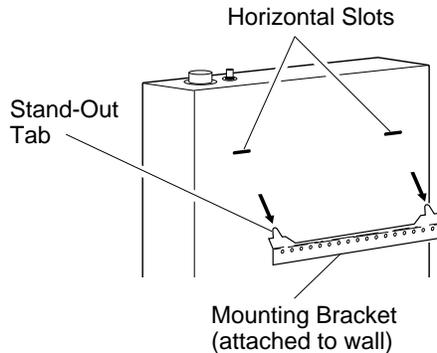
Figure 14 - Mounting Heater Onto Mounting Bracket
