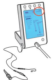
ENDOAce® automatically starts at the entrance of the canal when the tip of the instrument makes contact with the dentin (except MANUAL PROG 00). For a manual start, press the RUN/STOP button. In each case, the motor stops as soon as the contact between the instrument and the canal is lost.
