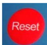
: Press this button to restart the machine. The laser head will first move back to zero point and then to original point.
