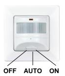
As with a regular light switch, the light may be switched OFF (left) or ON (right) permanently. The middle position will switch lighting automatically.
