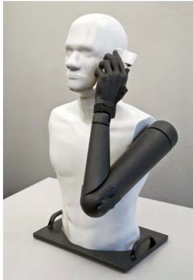
Figure 1.2: Torso phantom TORSO-X-V5.x with left arm phantom and left PDA hand phantom
