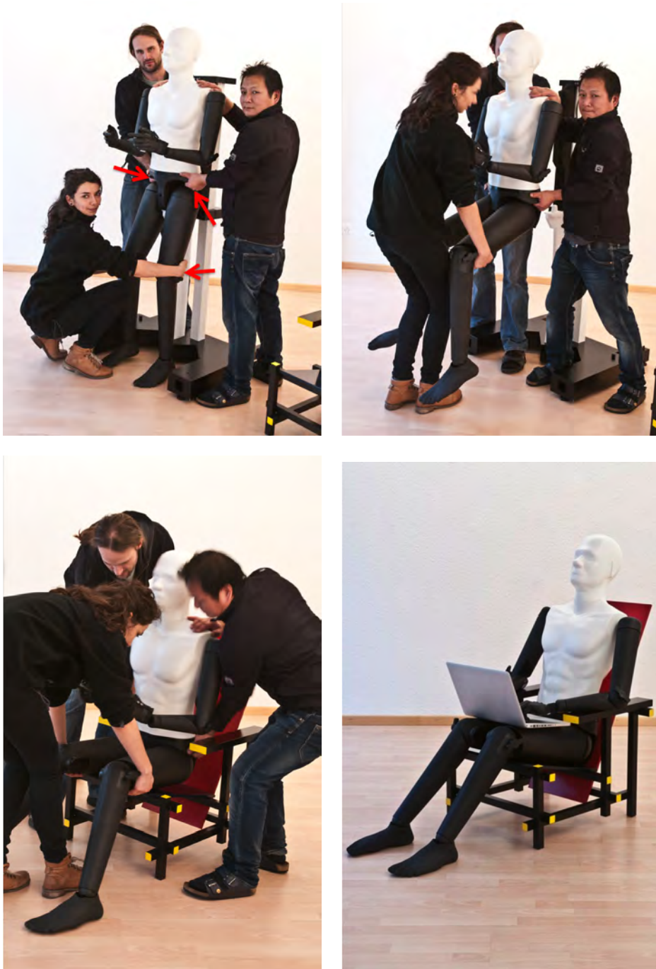
Figure 1.29: Recommended procedure to lift the whole-body phantom. Bottom right: Position with laptop on a chair
