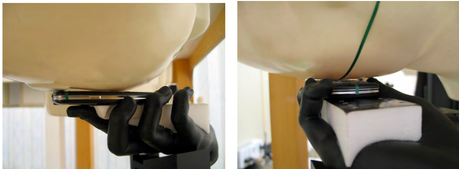
Figure B.1: Correct positioning. The DUT is in the cheek position and the back of the DUT is in good contact with the hand phantom spacer
