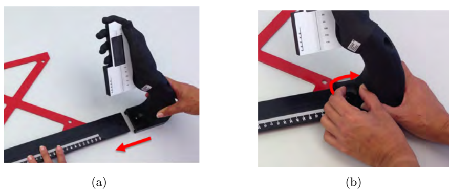
Figure 9.6: (a) Mounting the right hand to the fixture and (b) fixing the knob.
