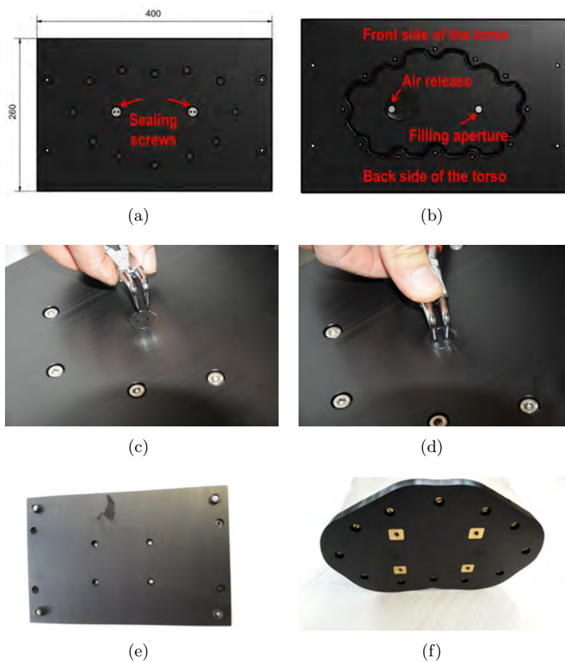
Figure 1.5: (a) The outer and (b) inner surfaces of the bottom plate, (c)-(d) removing both screws using pliers, (e) holder plate for new Torso designs (d) bottom plate for new Torso designs
