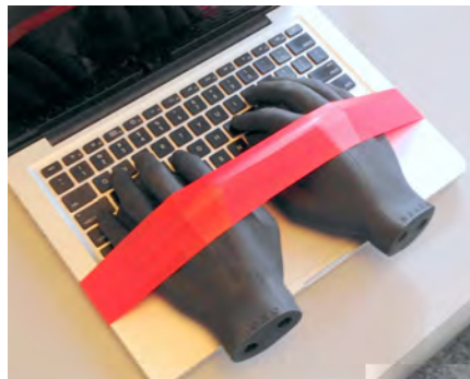
Figure 11.7: Fixing hands to the DUT for vertical rotation.
