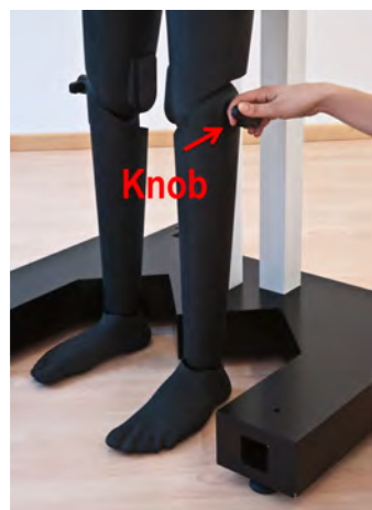
Figure 1.21: The knob on the knee to adjust the leg position
