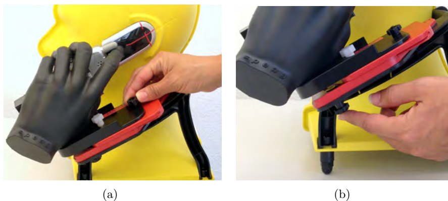
Figure 5.7: (a) Mounting the hand on the fixture/positioner using the screw at top; (b) loosening the screw at the bottom to rotate it
