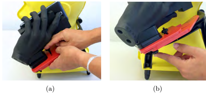
Figure 7.6: (a) Mounting the hand on the fixture/positioner using the screw at top; (b) loosening the screw at the bottom to rotate it
