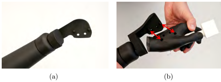
Figure 1.14: Mounting PDA hand phantom to PDA hand adapter
