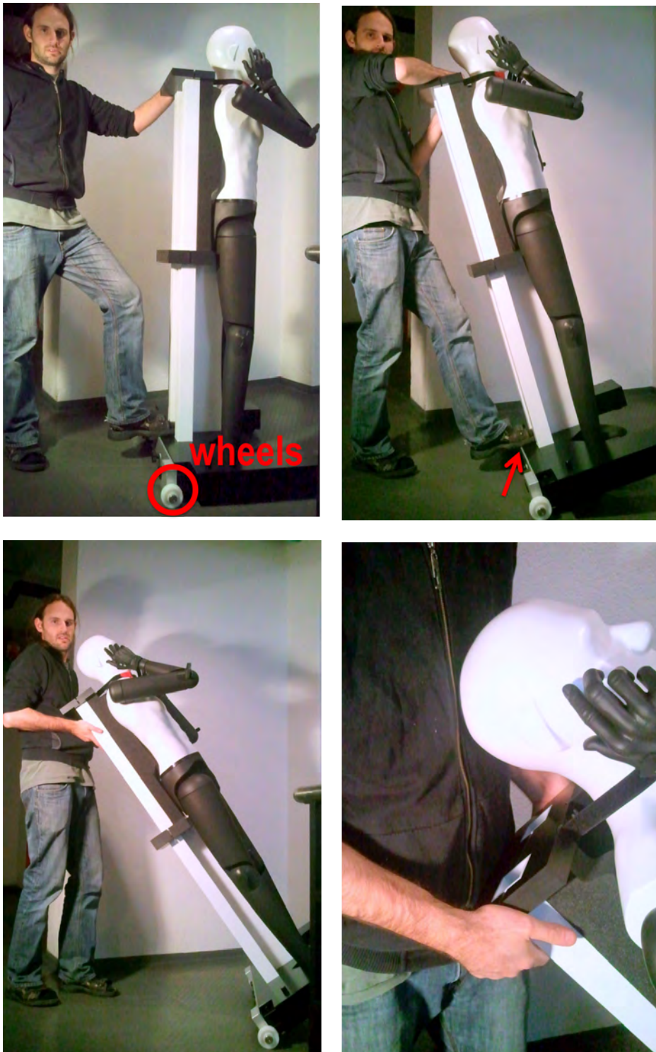
Figure 1.28: STAND-V5.x used as a dolly to transport the whole-body phantom
