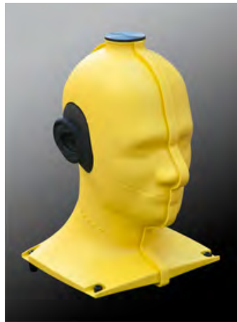
Figure 3.1: SAM-V4.5BSE Head Phantom with anatomically correct lossy Ears with ear canal
