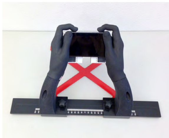
Figure 10.3: SHO-FX-HOTV4 - SHO Fixture X for Hand-Only-Testing V4 with right and left wrists (SHO-RTHG/LTHG-DWV4), hands, and DUT
