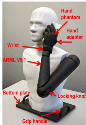
Figure 1.3: Torso phantom TORSO-X-V5.x parts
