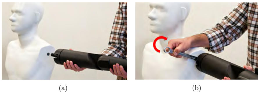
Figure 1.11: Mounting the arm into the torso manually and then tightening with a 20 mm wrench
