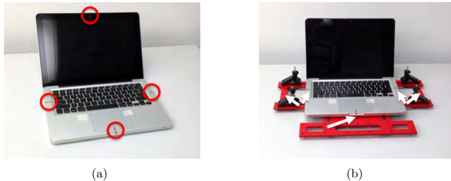
Figure 11.10: (a) Marking the edges of the geometric center on the DUT and (b) aligning with the fixture.
