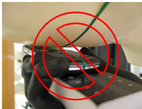
Figure B.3: Incorrect positioning. The DUT is not in the correct cheek position. For thin phones, the thumb of the hand phantom will make contact with the Twin SAM phantom before the DUT is in the cheek position. Hand phantom fingers are flexible and should be moved slightly to obtain correct cheek position.
