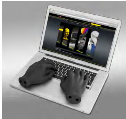
Figure 11.3: SHO-V2/3LLAP and SHO-V2/3RLAP hand phantoms positioned on a laptop device.
