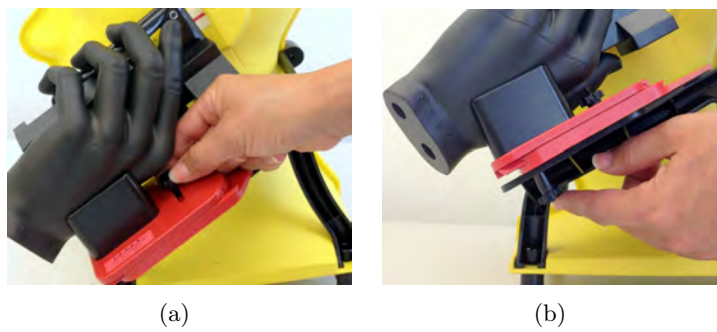
Figure 6.7: (a) Mounting the hand on the fixture/positioner using the screw at top; (b) loosening the screw at the bottom to rotate it
