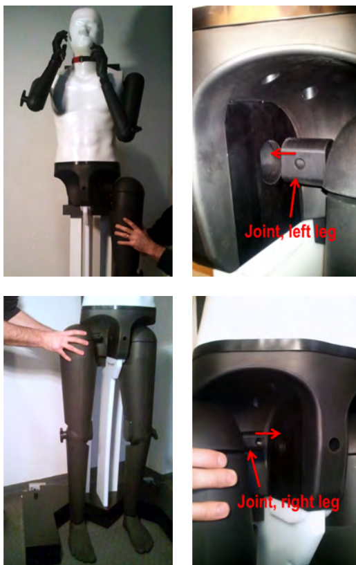
Figure 1.22: Attaching the leg to the buttocks phantom. IMPORTANT: Left leg mounted first
