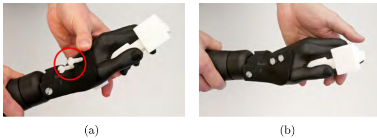
Figure 1.15: Fixing the PDA hand phantom by tightening 61 mm screws
