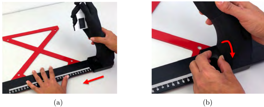
Figure 10.6: (a) Mounting the right hand to the fixture and (b) fixing the knob.
