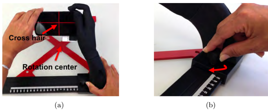
Figure 10.9: (a) Aligning the cross hair with the rotation center and (b) tightening the knob.
