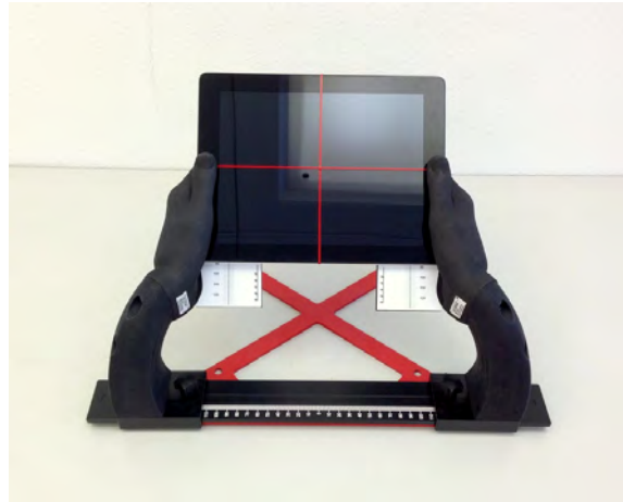
Figure 9.3: SHO-FX-HOTV4 - SHO Fixture X for Hand-Only-Testing V4 with right and left wrists (SHO-RTAB/LTAB-DWV4), hands, and DUT
