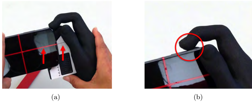
Figure 10.8: (a) Aligning the display center line with the spacer marker (b) index finger presses on the upper edge of the device.
