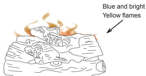
Figure 24 - Correct Burner Flame Pattern
