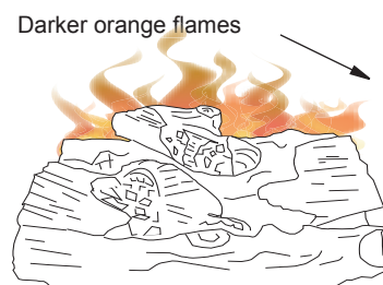
Figure 25 - Incorrect Burner Flame Pattern
