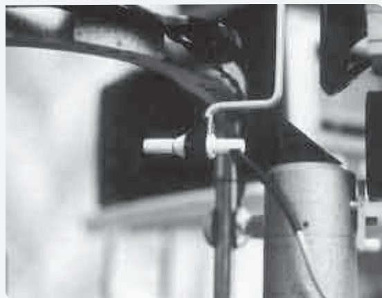
Figure 10-8. The small solid probe fits in the tonometer holder for A-scan biometry.
