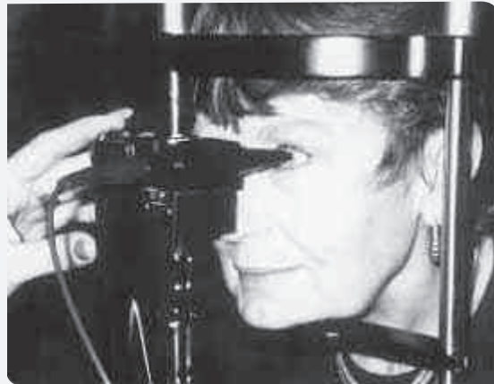
Figure 10-7. Contact A-scan biometry. The technician uses the joystick to align the probe with the patient's eye.
