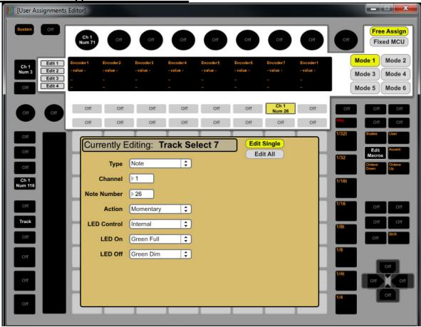
The User Assignments Editor allows you to edit the properties of controls not used by PXT-General (collectively referred to as *Global Controls* and displayed on a gray background) as well as the <u>8 Display Encoders</u>, <u>Track Selection and Track State Buttons</u>, Encoder Mode Buttons (Volume, Pan & Send, etc) and Display (collectively referred to as *Upper Controls* and displayed on a white background) when the <u>Scales Button</u> is turned off.
