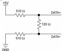
$120\Omega$  termination resistor always present between Data+ and Data-
