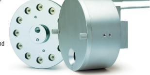
Crystal indexing is accomplished with a pneumatically driven mechanism. This pneumatically driven motor provides better thermal stability than competitive units using expensive in-vacuum, heat generating, electric motors. One-eighth inch water cooling tubes keep the sensor head thermally stable and allow flexibility in sensor placement.
