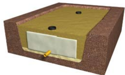
Step 8 - Lateral backfilling.
