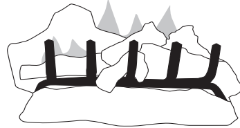
Figure 21 - Correct Burner Flame Pattern
