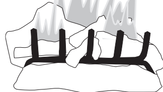
Figure 22 - Correct Burner Flame Pattern
