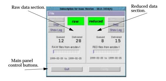
The dataSubscriber panel is divided into two sections each one controlling the acquisition of "raw" and "reduced" data:
