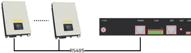
Fig. 6-2: Connect with the inverter
