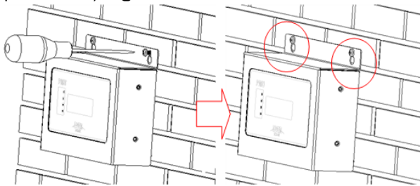
Fig. 5-4: Tighten the screws
