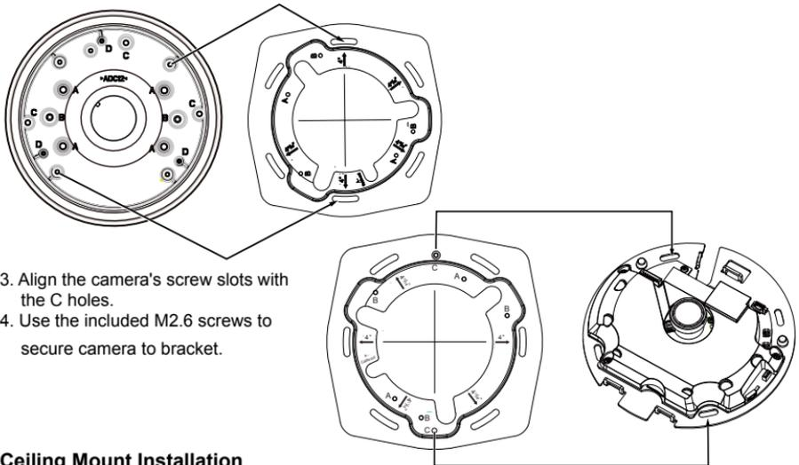
3. Align the camera's screw slots with the C holes.
