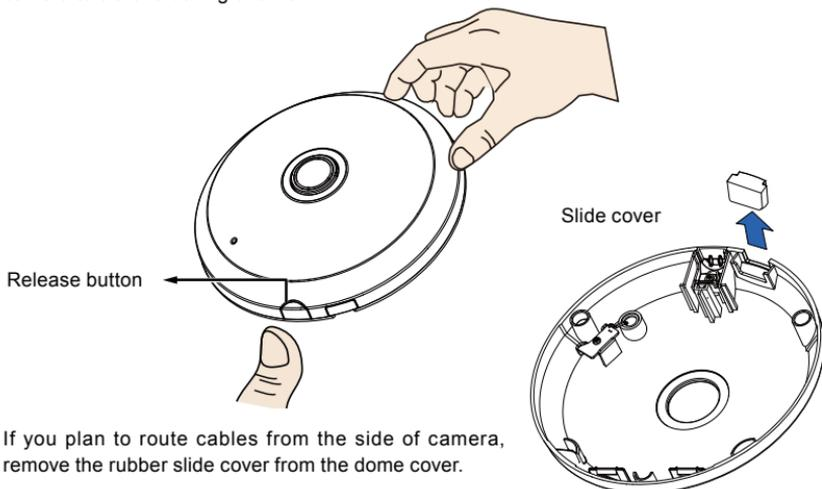
If you plan to route cables from the side of camera, remove the rubber slide cover from the dome cover.
