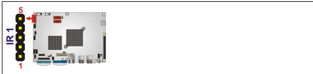
Figure 3-15: Infrared Connector Pinout Locations
