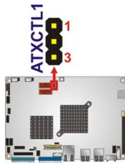
Figure 4-3: AT Power Select Jumper Location
