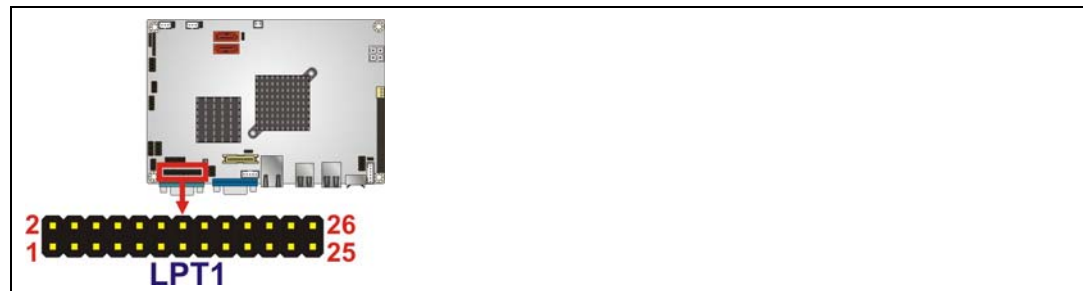
Figure 3-19: Parallel Port Connector Location
