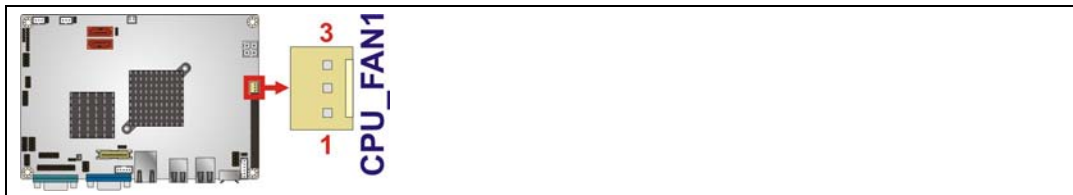
Figure 3-10: +12V Fan Connector Location
