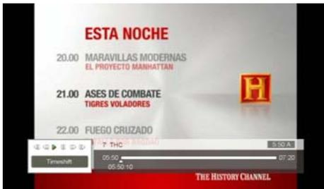
Time shifting enables you to pause the live signal and then continue watching the live signal from where the program was paused.
