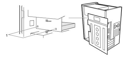
4 Remove the screws (1) on the right side of the floppy disk drive.
