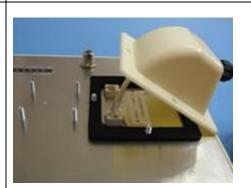
Plug the CAT5 cable into the Ethernet port, and fit the boot cover over the 4 studs and gasket. Secure with 4 kept nuts and tighten using a 3/8" wrench until the gasket is at least 50% compressed. Do not over tighten.
