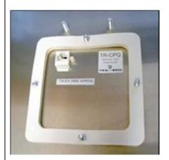
Place the gasket over the 4 studs around the Ethernet port.
