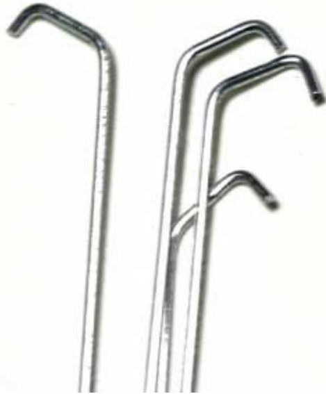
Figure 66: Close-up of hooks on the ground drop wires.
