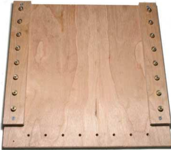
Figure 79: Wooden jig. Spacing between the holes and between the thumbscrews is 1.25" (3.17cm)
