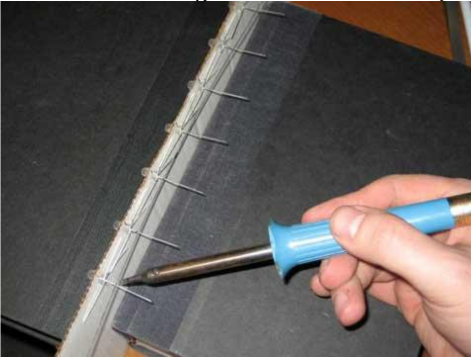
Figure 38: Soldering the LED strip on a cardboard jig.
