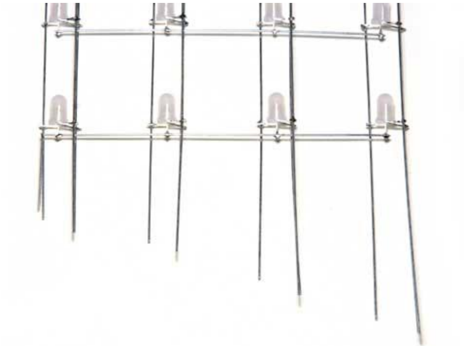
Figure 59: Cascading the drop wires for easier insertion.
