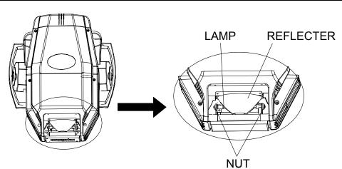
Lock the yoke before fitting/replacing the lamp.
