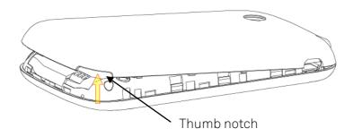
2. Insert your SIM card carefully into the SIM slot as shown:
